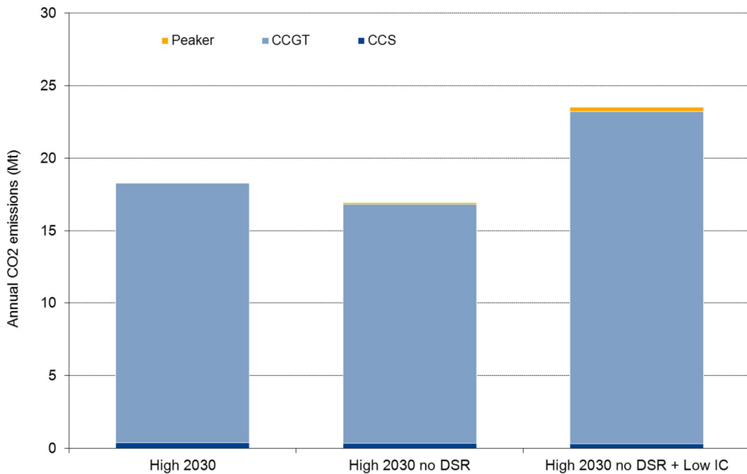
Figure 39 – CO 2 emissions by source in the High 2030 main scenario, no DSR variant and no DSR and low IC variant (MtCO 2 ) 136
